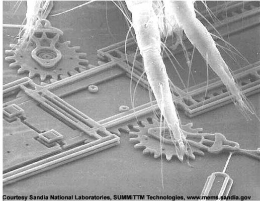
**Figure 1.** Spider mite with legs on a mirror drive assembly, illustrating the tininess of nanotechnology. *Credit:* Sandia National Laboratories, SUMMITM Technologies, <http://mems.sandia.gov/scripts/images.asp>
